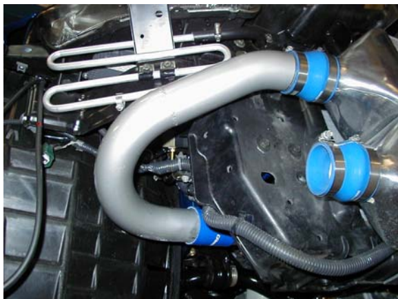
Right side turbo I-2 to the intercooler
