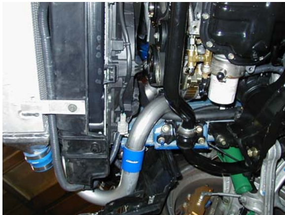
Right side turbo (C-1) to the Intercooler intercooler
